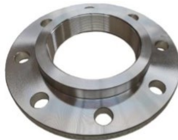
SS316 FLANGE - TABLE E - BOSSED SCREWED BSP
